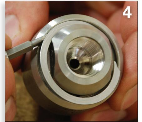
Once that is accomplished, gently rotate the tool while continuing to slide the screwdriver along, lifting the retaining ring out of the groove until it pops out completely. The ring comes off similar to a key sliding off a set of car keys.
