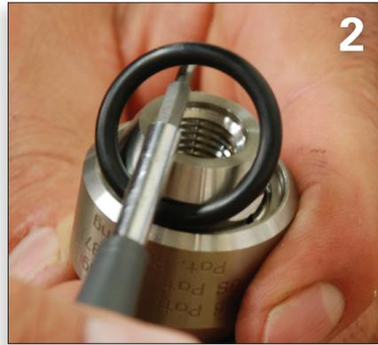
First, flip the tool over so the inlet nut is facing up. Use your flat-head screwdriver to pry off the O-ring from the inlet nut. Set the O-ring aside. With the O-ring off it will expose the retaining ring that keeps the inlet nut from sliding out of the body.
