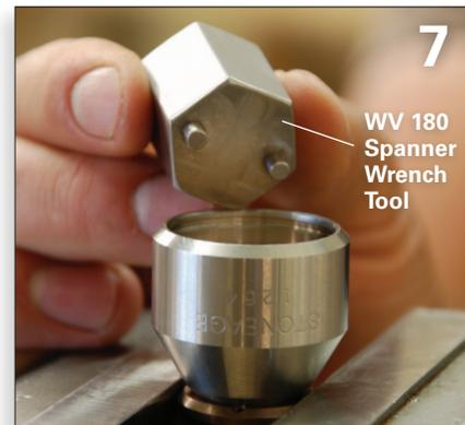
Place the body into a vice with the head down. There are two wrench flats on either side of the head. Make certain the flats are positioned properly in the vice. Next, take the WV 180 (spanner wrench tool shown above) and set it into the two holes in the brass shaft.
