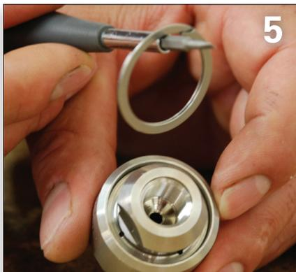
When completely out of the groove the retaining ring will look like this. Set it aside temporarily for re-assembly later.
