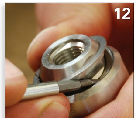
The last two steps are to re-mount the retaining ring and finally, slide the o-ring on to the inlet nut. Your **WV-P4™** disassembly and cleaning procedure is now complete. The process can be handled easily in the field or the shop. Total time to complete the cleaning is approximately 15-20 minutes.
