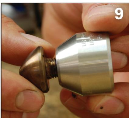
Finish unscrewing the head by hand. Remove the head and set aside. Make certain the head is clean and the drilled nozzles are free of debris. If necessary use a straight pin to clean out the drilled orifices.
