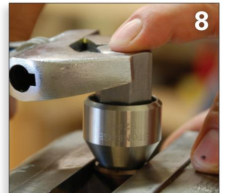
With your index finger applying downward pressure on the WV 180 spanner wrench, use a crescent wrench to loosen the shaft from the head in the vice. When reversing this step in re-assembly, do not overtighten the head into the shaft. 100 inch-pounds of torque is sufficient.
