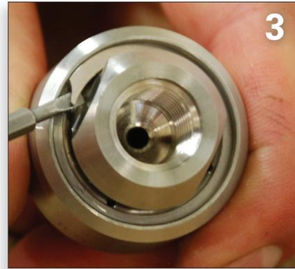
The retaining ring sits in a groove on the inside of the body. To remove the retaining ring locate the end of the ring and, with a flat-head screwdriver, separate the retaining ring by lifting the end out of the groove as shown above.
