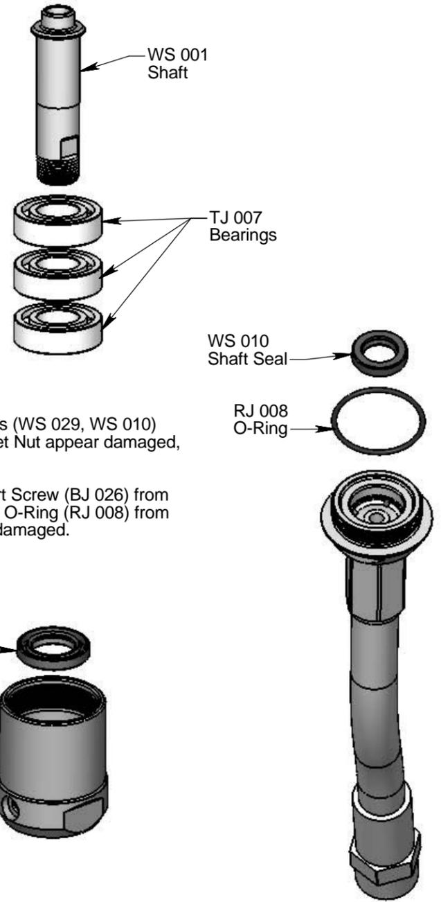
7. If Shaft Seals (WS 029, WS 010) in Body and Inlet Nut appear damaged, remove them.
