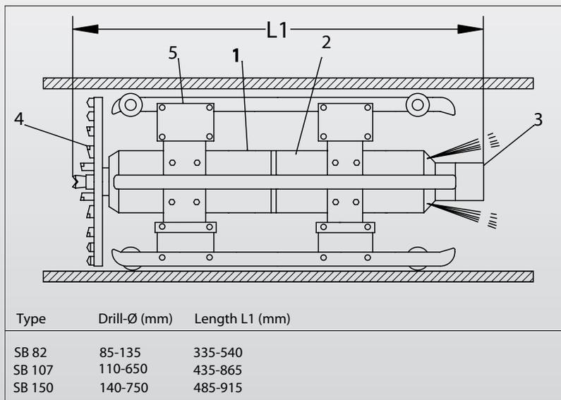
The six changeable jets (3), provide the machine with the propulsion to reach the problem area.
